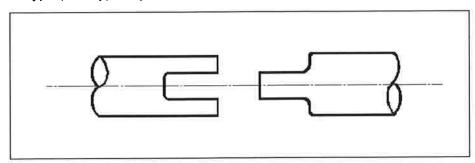
As the pump shaft (and the flattened end) is hardened, if the other half of the joint is of low hardness it will wear and may result in dry-running of the pump.
