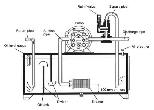
• Ensure that the pipe is supported with brackets to prevent its weight being applied to the pump.
